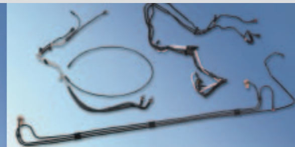
FLUID TRANSFER TUBING Dana engineers employ materials in innovative ways for chassis fluid-transfer tubing. Rubber, plastic, and metal are used separately or in combination to reduce weight with no compromise in performance or durability. Where applicable, tubing lines are engineered to reduce evaporative emissions or fluid-borne noise.
