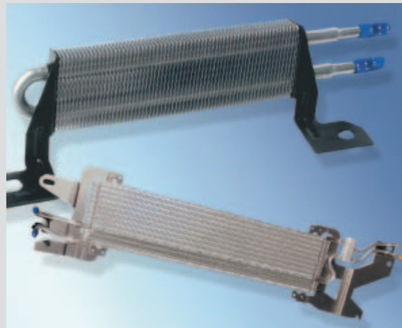
POWER STEERING OIL COOLERS Dana's innovative oil coolers are designed to minimize leakage and loss of assist by ensuring that fluid temperatures never exceed the specifications of hoses and seals in the pump – the primary cause of failure. Thermal valves, turbulators, and various oil-side enhancements all improve drivability and durability.
