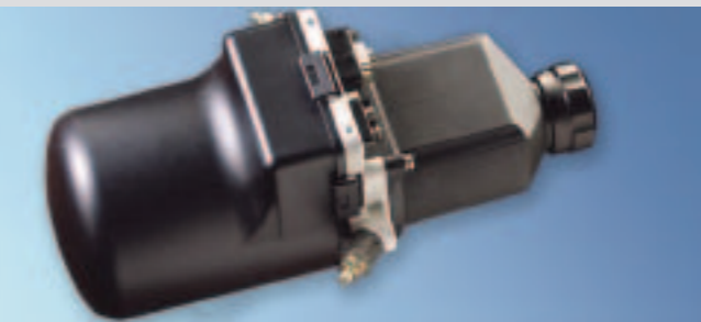
POWER PACK Dana power packs provide a wide range of solutions for electric hydraulic steering applications. Dana has extensive experience with DC brushless motors, high-efficiency pumps, and hydraulic systems. Power packs range from 500 to 5,000 watts with streamlined packaging that includes motor, control, and pump reservoir.
