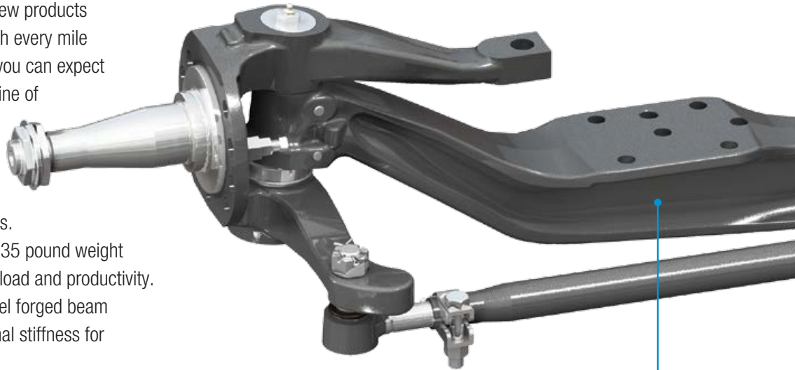
Lightweight beam available in standard and wide beam widths
